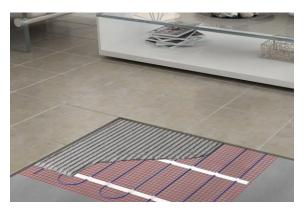
Generally associated with tiled or stone floors, underfloor heating can also be fitted in a carpeted conservatory. It can run on a pumped water system or a dry electric system. The downside of having an underfloor heating system is that compared to most other methods, it could turn out to be a little more expensive to install. It also means digging up and installing pipes below your conservatory floor. Underfloor heating would be a good option if you're thinking of having a
