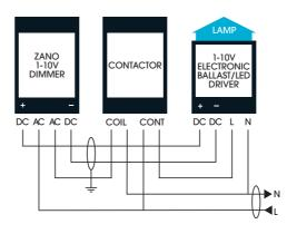
Installation converting from 1-10V to DSI
