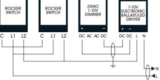
$\perp$  Screened cable at least 0.75m<sup>2</sup>. The screened cable must be used for + and – connections. The screening should be earthed only at one end.
