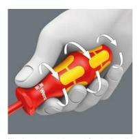
The hard materials used for the handle ensure rapid hand repositioning, without any danger of the skin "sticking" to the handle. The softer "anti-slip" zones enable the low-loss transfer of high forces – resulting in less screwdriving effort being required.
