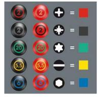
"Take it easy" tool finder: colour coding according to profile and size stamp. This enables faster and more reliable selection of the correct tool from the tool case.
