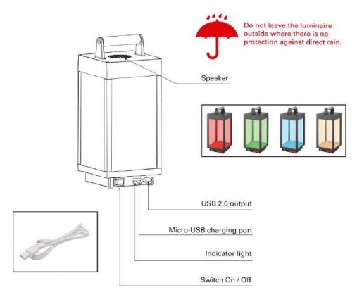
USB 2.0 output: Allows a smartphone to be charged. This, however, affects the battery life of the fixture.
