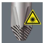
A precisely-focused laser creates a sharp-edged surface structure. This laser treatment results in an edge hardness of up to 1000 HV 0.3. Wera Lasertip "bites" itself into the screw head and prevents any slips out of the recess. It is available for screwdrivers for slotted, Phillips and Pozidriv screws.
