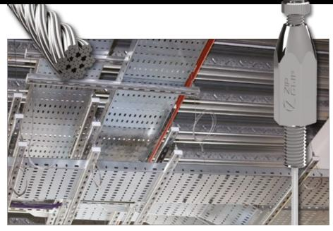
THE M8 AND M10 STRUT-LOCK SYSTEMS are used to support HVAC and M&E services from the S-RANGE and Y-RANGE of Zip-Clip wire supports respectively. The devices are typically installed into profile channel which can then be hung from a wire suspension.
