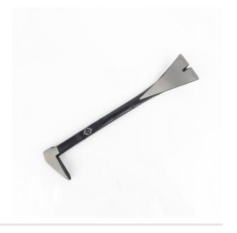
Features & Benefits Hot forged from carbon steel alloy, hardened for strength and durability. 46mm wide tip for precise removal with minimal damage. Flat heel for striking with a hammer.
