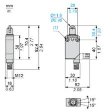
(1) 2 fixing holes Ø 4.2 mm, counterbored Ø 8 mm by 4 mm deep.
