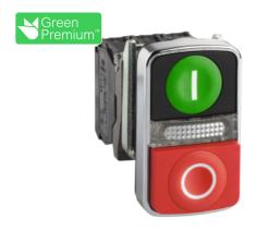
Illuminated double-headed push button, metal, Ø22, 1 green flush I + 1 pilot light + 1 red projecting O, 1 NO + 1 NC
