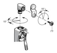
(1) Tightening torque (Min: 1) (Max: 1.5)
