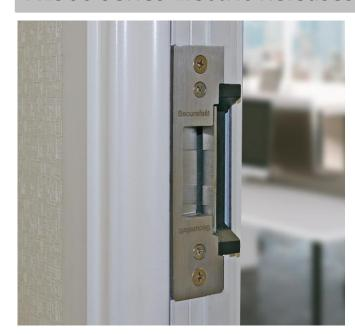
The AL900 series electric releases are an ANSI style door release, complete with stainless steel short or long faceplates for use in metal or timber frame applications. The electric release is designed to work with most leading brand mortice night latch locks.
