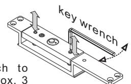
Using supplied key wrench to adjust armature plate to approx. 3 mm of gap between magnet and armature.
