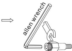
Use the allen wrench. To slowly tighten the Blind Nut. (Don't turning over)
