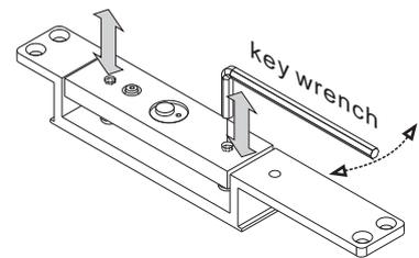
Using supplied key wrench to adjust armature plate to approx. 3 mm of gap between magnet and armature.
