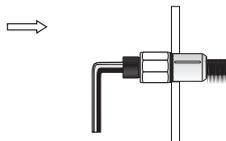
This compress the Blind Nut so that it remains permanently fixed in the frame.
