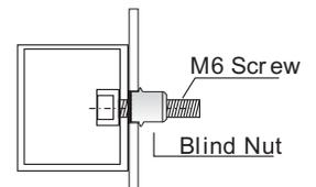
Use M6 Screws fixing SMB-001 brackets.
