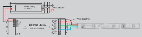
2) Receiver Connection Diagram for Multiple Units
