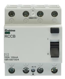
Four Pole RCCB, 100A 100mA, Type AC, For use with Crabtree Loadstar distribution boards, For incoming options can be used with 18LK125 connection kit
