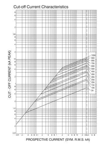
Designed for use in conventional house service cut-outs, ASTA Certified and in accordance with BS1361: 1985. The ordering code is Rating followed by KR85 e.g. 40KR85. Carton quantity - 20 all ratings. Dimensional details in mm.
