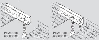
Tray widths up to 225 mm Two quick bolt fasteners per coupler
