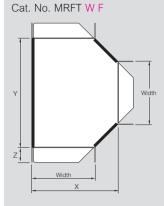
X = Length of fitting from each end (excluding integral coupler) Y = Length of fitting from each end (excluding integral coupler)
