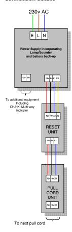
Use 'intruder alarm' type stranded cable for interlink wiring. DO NOT USE 'TWIN & EARTH or other rigid cable types!
