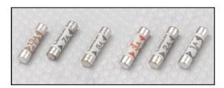
Lawson Type "PL" fuse-links are intended primarily for use in domestic plugs but may also be installed in appropriate single-phase installations with fault levels up to 6kA and have nominal dimensions of 6.3 x 25.4mm.
