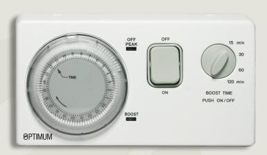
The Optimum Ecosave is a mechanical 24 hour multi tariff timeswitch used to control 3KW electric immersion heater elements for timing of water heating during low tariff electricity supply periods, and a boost function selectable for 15, 30, 60 or 120 minutes for peak tariff periods. Suitable for use in dry rooms only! Do not install in the vicinity of devices which generate inductive discharges (motors, transformers, etc.)!
