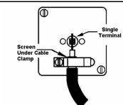
Each coaxial cable should be connected to the appropriate terminal as shown.
