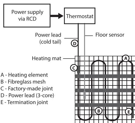
of the bathroom, as close to the installation as possible. Rointe thermostats are rated up to 16A. For larger installations exceeding 16A multiple thermostats or a suitable contactor will be required. For further advice contact Rointe.
