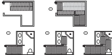
**NOTE:** When laying two or more heating mats, ensure the cold tails reach the thermostat.
