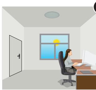
The sensor switches off the light whenever natural light exceeds pre-set daylight threshold, even with presence.
