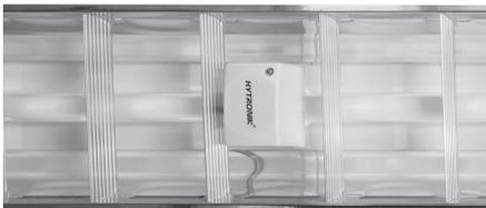
Most of the linear office lights have metal louvre, where microwave cannot penetrate through. An easy alternative solution is to use this detached sensor antenna head, grip on the T5 and T8 tube, and put the sensor main body behind the metal louvre, together with the ballast or driver.
