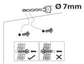
Fix the U bracket to the wall using the correct screws for the wall plugs being used. Note: Ensure that when you mount this, the slots at the end of the bracket open upwards to allow you to easily attach and secure the floodlight when ready.
