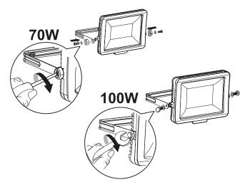
Pass the supply cable through the holes(s) provided in the backplate ensuring that a cable gland, grommet or sealing compound is used to maintain the IP rating of the floodlight.
