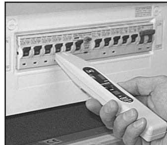
Figure 4. Correct The receiver must be held in this orientation in relation to the breaker to find the correct fuse/circuit breaker. If the individual breakers were horizontal, the receiver would have to be rotated through 90° (in either direction).
