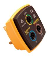
Speed up 17th Edition, Part P and periodic testing of electrical installations with this plug-in adaptor. The SB13 enables safe and fast testing at socket outlets without the need to remove the socket faceplate from the wall. This saves time when taking R2 and R1+R2 measurements as well as voltage measurements.
