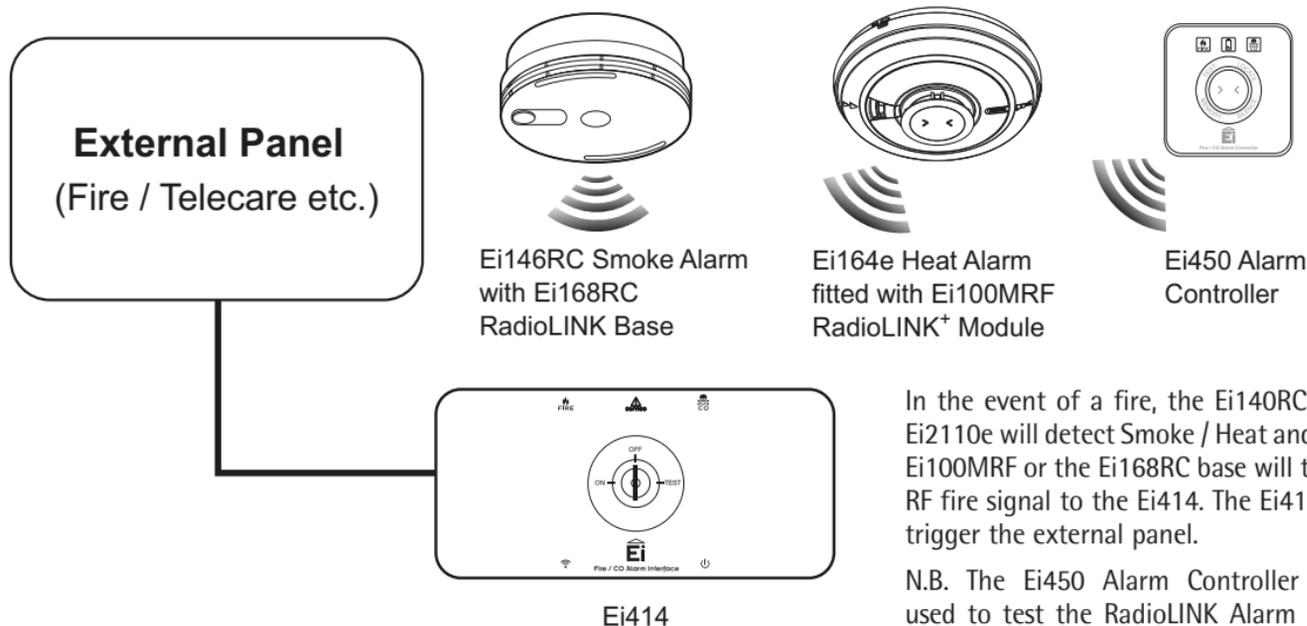
In the event of a fire, the Ei140RC / Ei160e / Ei2110e will detect Smoke / Heat and either the Ei100MRF or the Ei168RC base will transmit an RF fire signal to the Ei414. The Ei414 will then trigger the external panel.
