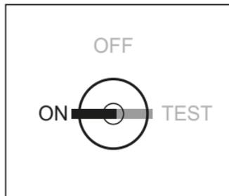
In the 'ON' position the Ei414 responds to a fire alarm signal (activates the fire relay) or to a CO alarm signal (activates the CO relay).
