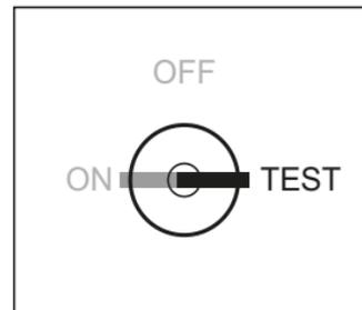
In the 'TEST' position the Ei414 responds to a button test signal (will activate the fire or the CO relay depending on the unit that was button tested).
