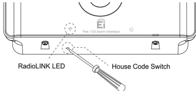
House Code all other RadioLINK Alarms and devices in the system. Consult the instruction manuals on how to House Code the Alarms and devices. It is essential that each individual Alarm / device is put into House Code mode in it's actual location.
