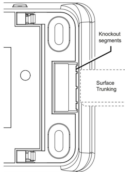
Rear View: optional wiring using surface trunking
