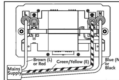
N.B. Green/yellow earth wire may be connected to either earth terminal. Wiring insulation tests should be completed before setting the PowerBreaker RCD Socket to avoid misleading instrument readings and possible internal damage to the unit.
