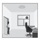
With ambient light more than the setting value, the lamp does not switch on when someone enters the room.
