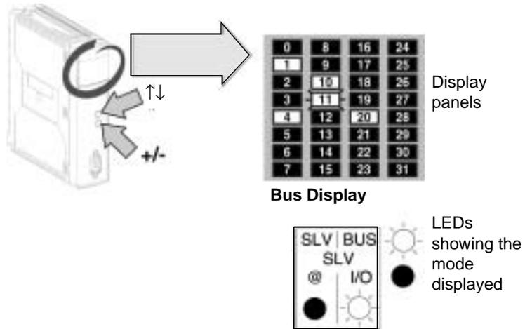
The image of the AS-i network is displayed on the entire display panel. Each LED represents an AS-i bus slave address.
