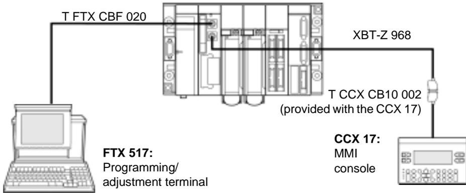
**Note:** Each connected terminal can be disconnected without disrupting the operation of the other. For an Atrium PLC or if the processor only has one terminal port, this type of connection can be made by using a **TSX P ACC01** (See *TSX P ACC 01 device, p. 47*) device.
