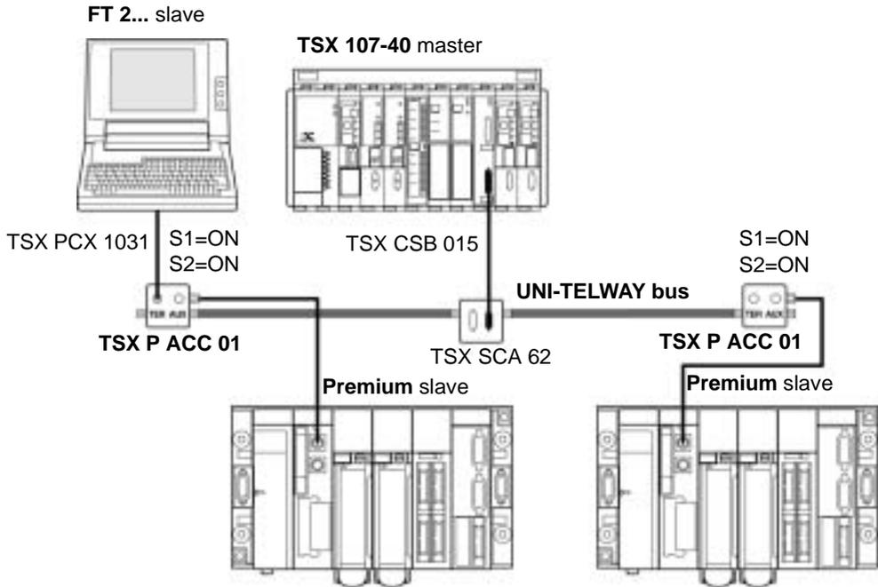
**Note:** To install **TSX SCA 50** and **TSX SCA 62** devices, consult the TSX DG UTW manual: *UNI-TELWAY Bus communication*
