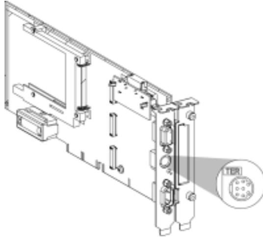
This connector is used to supply power to a device which does not have its own power supply (connecting cable converter RS 485/RS 232, insulating device **TSX P ACC 01** (See *TSX P ACC 01 device, p. 47*), etc).
