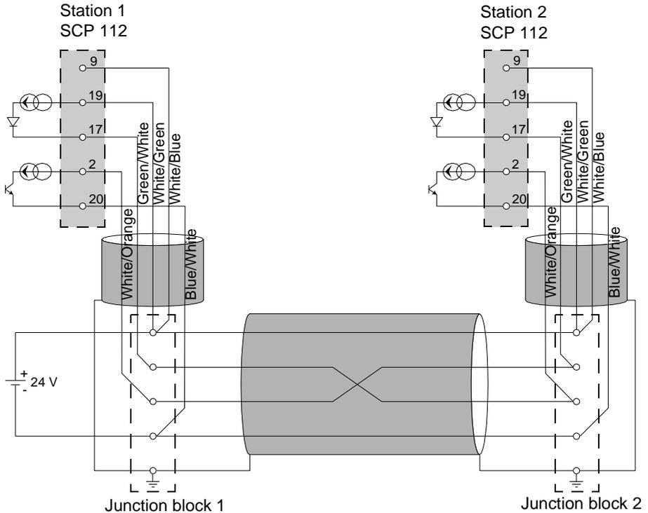
**Note: Important:** the cable shielding must be connected at the shortest point in the junction blocks.
