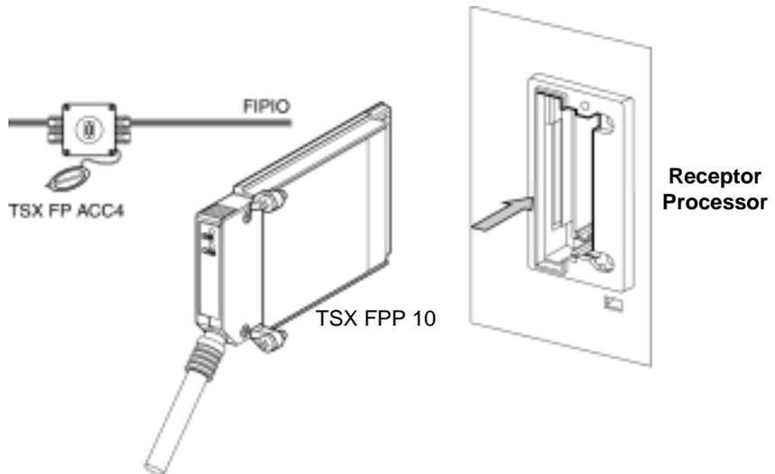
**Note: Important:** cables (**TSX FP CG 010/030**) are connected and disconnected from the PCMCIA card only **when power is switched off**.
