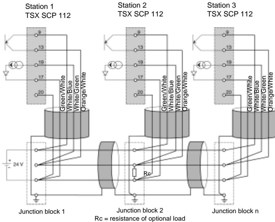
**Note: Important:** the cable shielding must be connected at the shortest point in the junction blocks.
