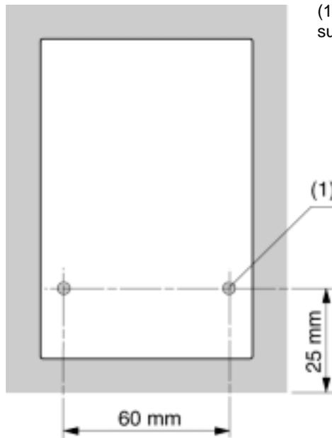
(1) Screw hole diameter must be suitable for M4 screw
