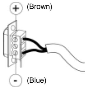
In the special event that a shielded cable is used, this should be connected to the central terminal.
