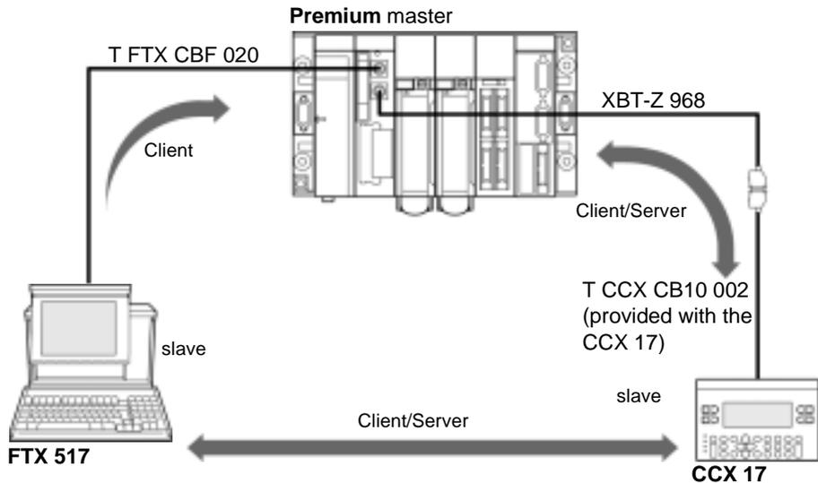
**Note:** In the case of an Atrium station where the processor only has one terminal port, this type of connection can be made by using a **TSX P ACC 01**
