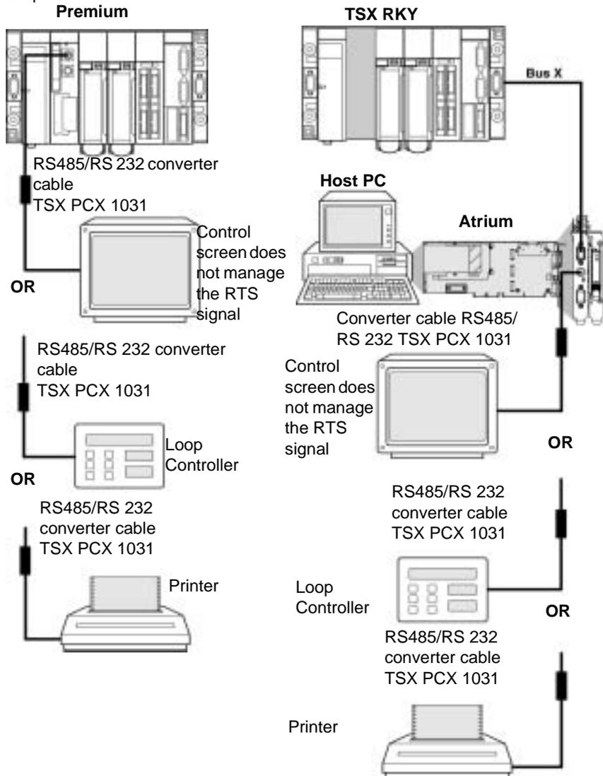
**Note:** In order to ensure all types of connection **TSX PCX 1031** and **TSX PCX 1130** cables are delivered with adapters:
