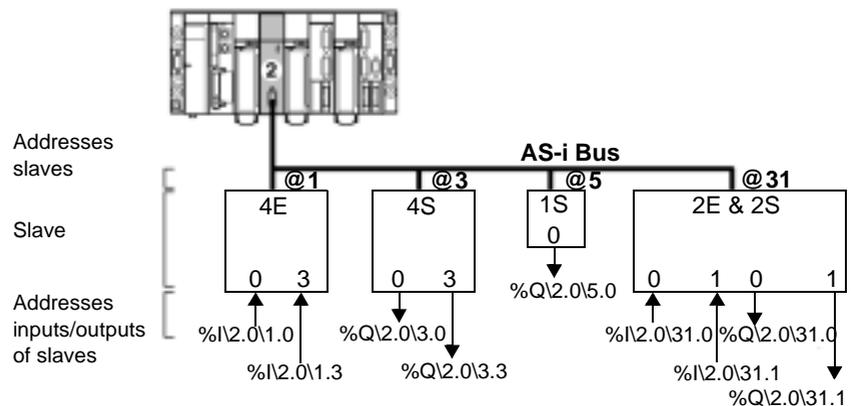
**Note:** The physical address of an AS-i slave is programmed by the portable console **XZM C11**
