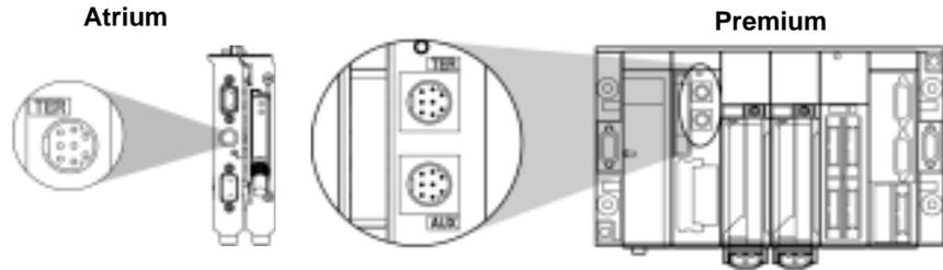
**Note:** For Premium PLCs with two connectors (TER and AUX), the operating mode defined in configuration (master UNI-TELWAY, slave UNI-TELWAY, character mode) is the same for both connectors.
