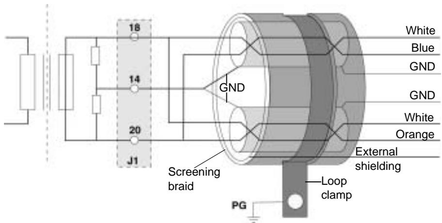
**Note: Important:** The cable's main shielding is grounded using a metal clamp in contact with the screening braid, which itself is fixed to the frame supporting the rack.
