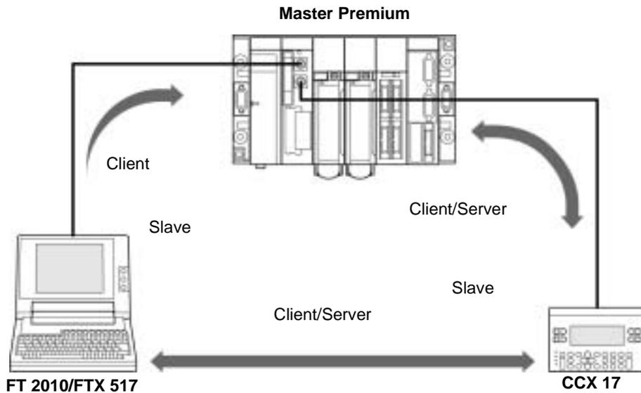
**Note:** When using an Atrium PLC or if the processor only has one terminal port, this type of connection can be made by using a **TSX P ACC 01 device**. (See *TSX P ACC 01 device*, p. 47)
