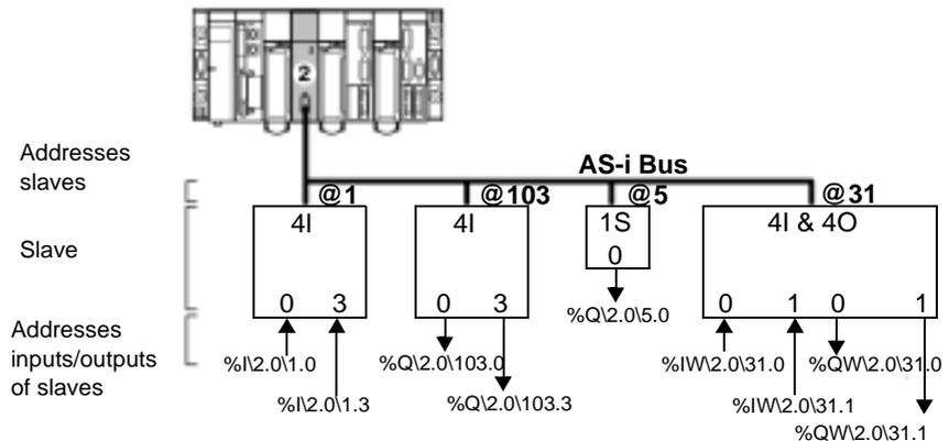
**Note:** The physical address of an AS-i slave is programmed by the **XZM C11** portable console.
