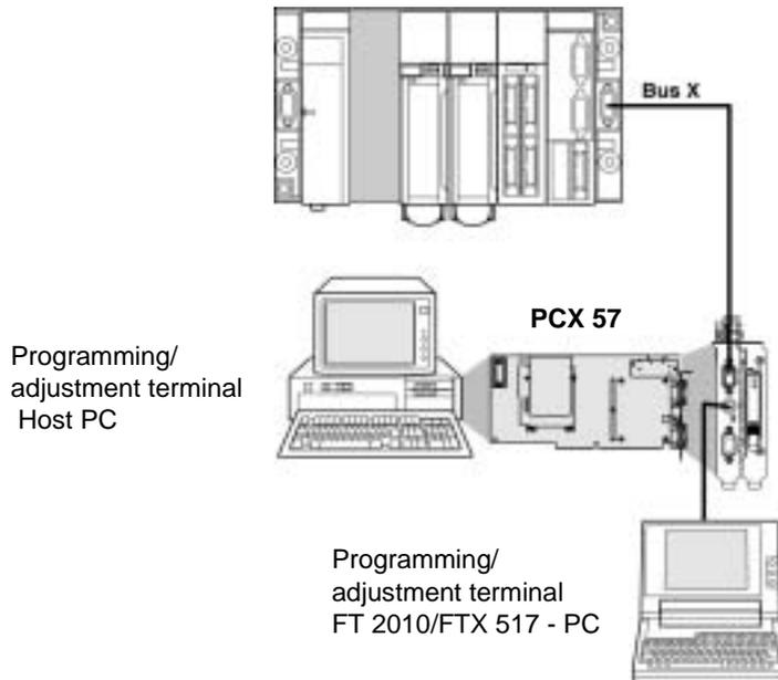
**Note:** When using an Atrium Station, the programming terminal is generally the PC which accepts the PCX 57 processor. However, as for a Premium station, the programming terminal can also be a PC type terminal connected to the processor port.
