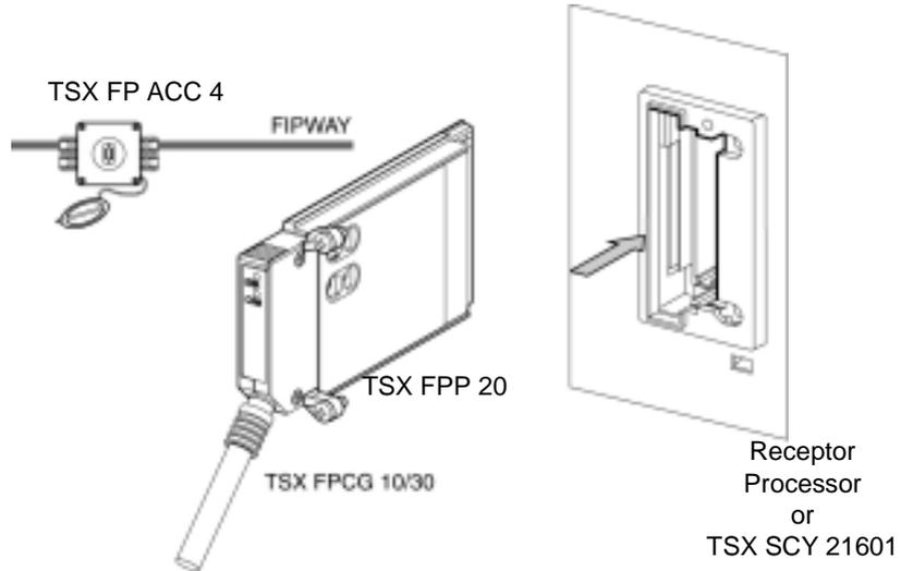
**Note: Important: TSX FP CG 010/030** cables connect and disconnect from the PCMCIA card only **when power is switched off**.
