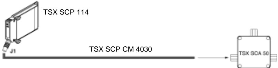
**Note:** The length of the cable used (3 m), makes it possible to link a device to a **TSX SCA 50** connection device located within a 3 meter radius of the card. This length ensures connection inside a standard cabinet
