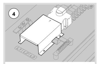
Refit the busbar shield and fit the direct connect shield
