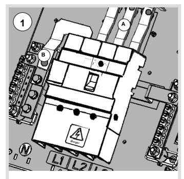
Fit the MCCB to the pan assembly with the fixings provided (do not tighten at this stage). Remove the  $3 \times M8$  coach bolts from the L1, L2 and L3 busbar. Fit the extension links (note the orientation of the links (**A**). Fit the  $3 \times M8$  Allen bolts (6mm Allen key). Do not tighten at this stage. Remove the neutral swing link from the board and fit the neutral connection between the MCCB and the neutral connection point (**B**).
