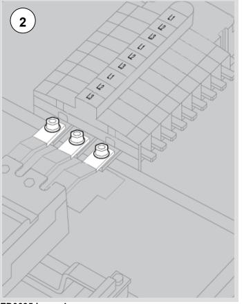
Connect the extension links to the busbar with the 3 x M8 coach bolts and the neutral connect using 1 x M8 coach bolt. Hand tighten at this stage.
