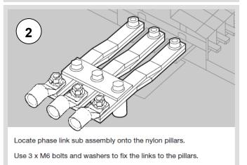
Use 3 x M8 bolts and washers to fix at busbar end.
