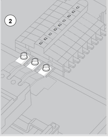
Fit the MCCB to the pan assembly with the fixings provided (do not tighten at this stage). Remove the  $3 \times M8$  coach bolts from the L1, L2 and L3 busbar. Fit the extension links (note the orientation of the links (**A**). Fit the  $3 \times M8$  Allen bolts (6mm Allen key). Do not tighten at this stage.
