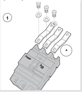
Connect the extension links to the busbar with the 3 x M8 coach bolts. Hand tighten at this stage.
