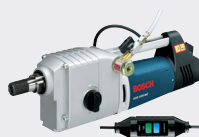
GDB 2500 WE Professional, 2500 W G 1/2" and 1 1/4" UNC toolholder (0 601 18P ...)
