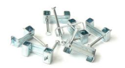
The Termination Technology brand of metal T&E clips provide an 18th Edition compliant solution to fixing T&E cables. Made with a simple yet effective design, our clips knock in to fix with a 4.5mm on all head. They are resistant to fire, corrosion, solvents and chemicals.
