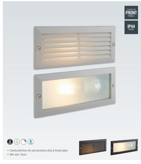
CODEDESCRIPTIONLAMPFINISHDIMENSIONSCUT OUT52213Eco plain & louvre IP44E27 GLS (required)Textured greyProj: 6mm H: 100mm W: 235mm85 x 226mm0L60ABEco plain & louvre IP44E27 GLS (required)Textured blackProj: 6mm H: 100mm W: 235mm85 x 226mm
