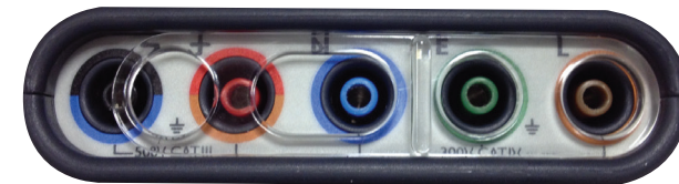
Fig.2 Interlock in position for RCD & Loop testing
