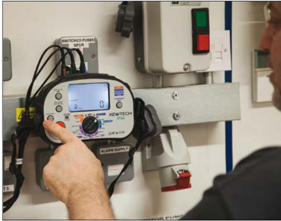
'Hands free' test button for continuous testing and a cleverly designed magnetic base; shown in action above.
