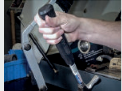
Nail extraction test for claw hammer
