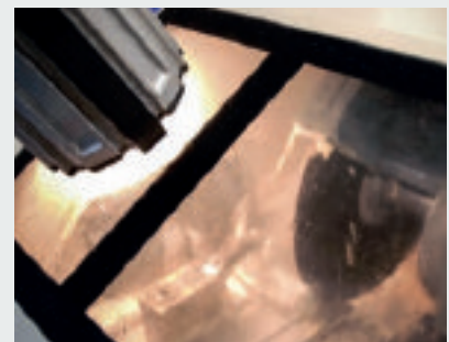
Hammer head is sliced to facilitate hardness testing of both the striking face and at 3mm depth
