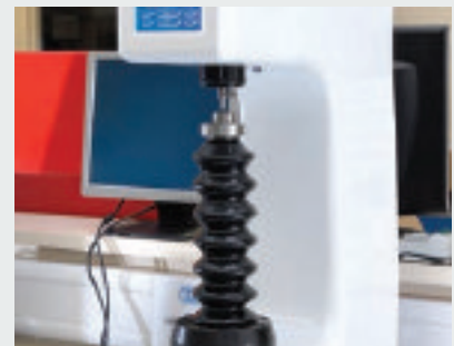
Measuring hardness of the striking face
