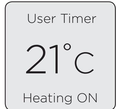
When the heater is in a timer profile and trying to achieve or maintain a room temperature, 'Heating On' will be displayed, otherwise, 'Heating Off' will be displayed. The words 'Heating On / Off' will not be displayed in a manual mode of operation.
