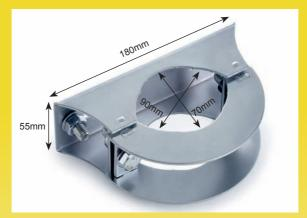
70-90mm adjustable pole bracket to carry one or two floodlights up to 100W LED / 400W Son fitting For one fitting: Fit floodlight directly onto the KRP11
