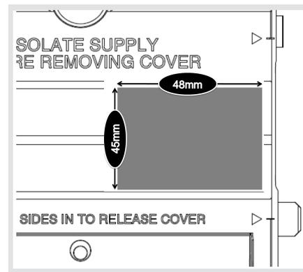
Mark the shroud ready for cutting out the aperture to allow the device to protrude through.
