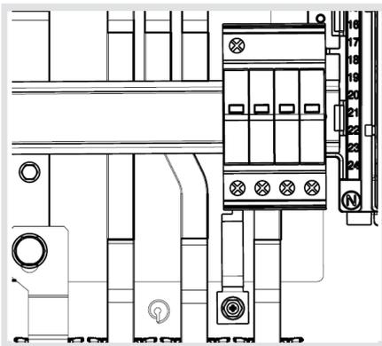
Clip surge protection device to din rail on the right hand side as shown & connect the copper earth link into the SPD and using the Hex head High Torque screw to the chassis at 5Nm
