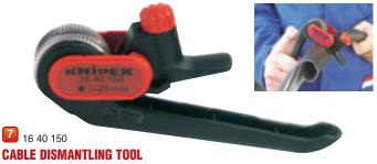
Professional Quality, for the removal of all layers of insulation on cables with diameters over 25mm. The cutting depth can be adjusted from 0-5mm depending on the insulation thickness. Cuts around or along insulation. Supplied in plastic storage case.
