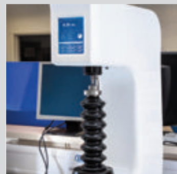
Measuring hardness of the striking face
