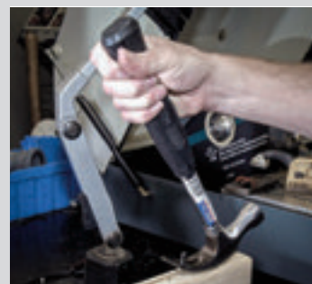
Nail extraction test for claw hammer
