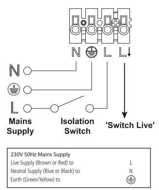
Note: the L↓terminal is a Switch Live "Live Output" for slave floodlights (when used in conjunction with the Timeguard LEDPROSLB-WH, PIRs or the LEDPROPCB-WH Photocell).
