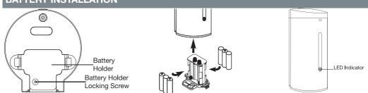
Prior to installing the ATC Dahlia Auto Dispenser on the wall, remove the battery holder from the base of the dispenser and install 6 good quality AA batteries; ensure the correct polarity in the battery holder. Once the dispenser is mounted and the batteries are installed correctly replace the battery holder into the dispenser and insert the battery holder locking screw and tighten.
