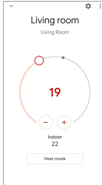
You can select the Heat mode, which is equivalent to MANUAL. The Comfort temperature is set, which can be modified. You can also set the ECO mode.
