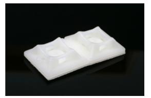
The Termination Technology range of self adhesive cable tie bases are available in a 20mm or 25mm version in black and natural. A coating of synthetic rubber on both sides of the foam base ensures high levels of tack and adhesion. Black mounts are ideal where applications are subject to sunlight and aggressive external conditions as they are UV resistant. Supplied in trade counter packs of 100
