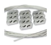
The Termination Technology range of catenary wire and grips are suitable for hanging lighting in high areas with a lower installation time compared to other methods. Self sustaining design with grips that use the weight of the installation to lock the retaining pin on the gripping wheel and hold securely in place. Available in a range of diameters and as a ready to use pack.
