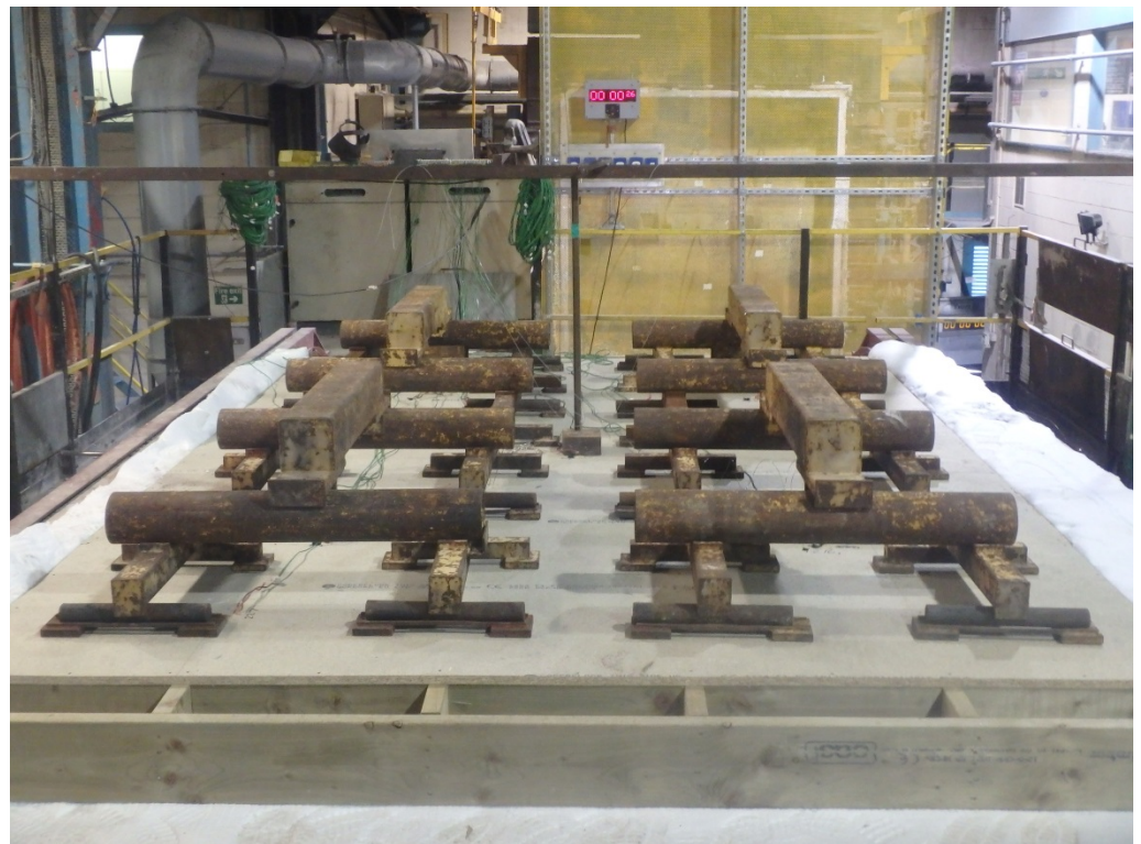
The unexposed face of the assembly prior to the start of the test
