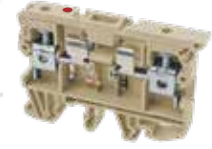
6 mm 2 Fuse Terminal Block with LED XX: 24AC/DC, 48AC/DC, 110AC/DC, 220AC/DC For 35 mm G and DIN Rail
