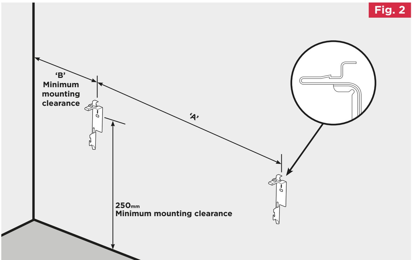
To mount the heater to the wall:
